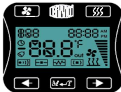
**[SSS]** - Turning the heating on or off – push
